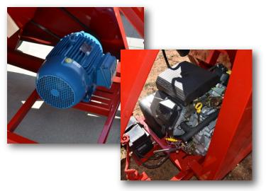
Savage Cleaners can be ordered with industrial grade electric motors or Kohler gas engines.
